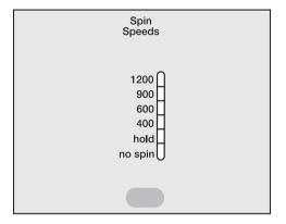
Press the "Spin" button until the indicator for the desired spin speed lights.
